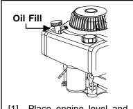
[1] Place engine level and clean around oil fill area.
